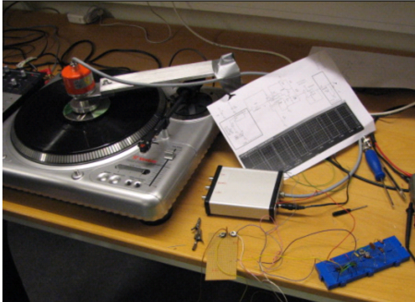
Figure 4. A sensor equipped turntable, with an interface circuit for the Toaster
